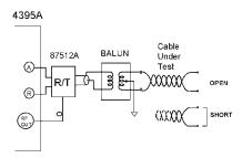
During the attenuation measurement a grounded shield should be used to isolate the two ends of the cable.
