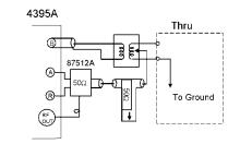
The following figure shows the setup configuration of Isolation calibration for LCL.
