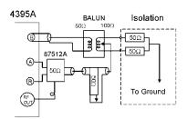
Since the impedance matching at the far end is very critical for LCL measurement, you have to choose the terminating resistance carefully. To ensure a good LCL measurement, the termination used here should have precise resistance value over the frequency range of interest. The recommended accuracy for the resistance is 0.01%.
